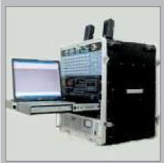
he UNESCO/ABU ■ "box" measuring around 55x50 cm contains a laptop, mixer, CD/cassette player and a 30W FM transmitter. The "box" can be used to produce radio programmes using a portable digital audio recorder, microphone inputs or other pre-recorded
